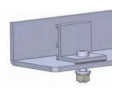
2) Connect the Angle Bracket to Rectangular Tube-Master with 8pcs U bolts, 16pcs M10 nuts, 16pcs spring washer, 16pcs washer as shown in the figure below.
